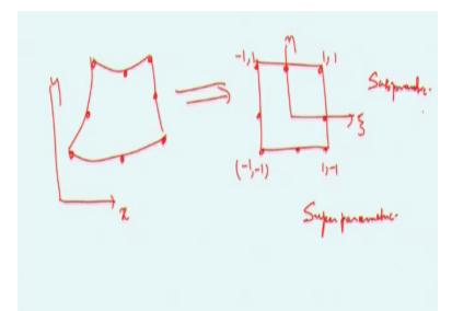
Suppose, we have an element we call this an element curved element having 8 nodes, which I write here, we map this onto a straight edged elements which is a perfect square, so this would be in basically xy co-ordinate system, whereas this would be in psi eta co-ordinate system. This is basically transformed to -1, -1, this is 1, -1, 1, 1 and this will be -1, 1.
