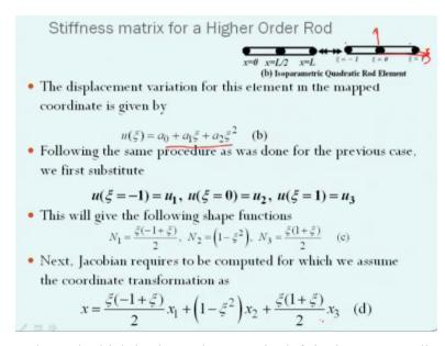
So this is a higher order rod which is shown here on the left is the xy co-ordinate system and the right is the psi co-ordinate system, so the origin is exactly here, so we have this psi in this direction, so psi=0 at the middle and it again the unit is equal to 2 varying from -1 to +1. So here we have 3 nodes, the nodes are located at x=0, x=L/2 and x=L in xy system and psi=0, psi=-1 and psi=+1 in the psi system. As I said once we are mapping it we will work only on the psi system.
