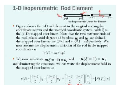
Let us now think about how we can actually formulate an isoparametric element, to demonstrate it let us take the simplest example that is the rod element, we had in the last lecture derived the stiffness matrix for the rod element. Now we will do the same using the isoparametric transformation. So the figure here shows a rod element which can have only 2 degrees of freedom that is you have u1 and u2.
