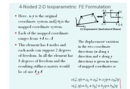
Now let us see how we can actually do a more complex by formulating the 2-D isoparametric finite element formulation, so you have a very arbitrary element which may be a quadrilateral in this quadrilateral we have straight edges of arbitrary shape, so to handle this in the conventional method becomes extremely difficult, this is the form of some kind of an arbitrary trapezium, so we mapped it to a completely a square of psi eta coordinates.
