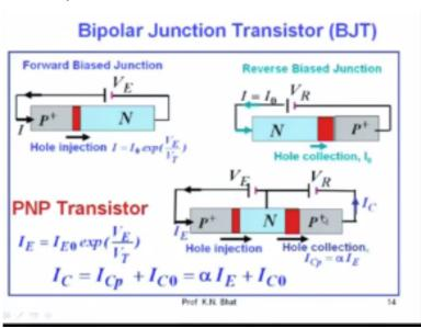
So, silicon you can go to about 150 degree centigrade without worrying about its operation, it will still work as a diode, you go to gallium arsenide, even go to 200, 250 centigrade, it will work as junction, okay, so what we will do now, we will quickly take a look at the bipolar junction transistor, I do not think I can go beyond bipolar junction transistor today and we finish up this junction transistor.
