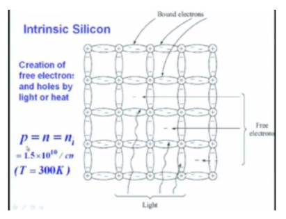
So, the electron tendency will be 0 and silicon will actually gave like an insulator at 0 degrees kelvin, okay. So, but in go to room; the room temperature, so what I showed you is intrinsic silicon, in the sense there are no impurities, purely it is silicon. Now, this intrinsic silicon at room temperature what happens is; some of these bonds, for example you can see there is one electron is missing from this.
