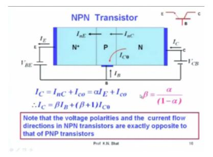
So, I can use it as an amplifier, okay. So, I can have NPN transistor or PNP transistor also okay, so these are the PNP transistor that this exactly same thing what happens is the forward bias junction injects current in the direction, emitter current flow is, you can see exactly opposite to the PNP transistor, collector current also is exactly opposite to the direction.
