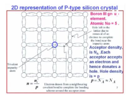
If it has moved away from atom far away whether there is net + charge there around that please remember that when you go to PN junction, so it is n type material. Now, the p type material, see instead of introducing phosphorous which is atomic number is 15, valence electron 5. I introduce boron; boron is a third group element in the periodic table and its atomic number is 5 which would be there will be 5; atomic number is 5.
