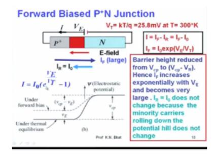
Now, let me see if I being instead of making this N side more positive and make P side more positive in the sense, originally it was VCP with + here, - here, I apply opposite velocity that is P side positive, N side negative like this; +=on the P side, so originally it was VCP like this with + here, - here, I apply + here, - which add some to that, so the voltage VE is applied, therefore the barrier height is reduced from VCP by VE.
