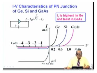
Generates a large number of electrons hole pairs which give rise to large current flow, which will be actually in the same direction as the reverse current flow always supply has to come from the battery, okay. Now, you can actually see the characteristics for different materials, for example, if I take germanium the characteristic is like this, like this is a forward, this is reverse telling you that I0 is very large for germanium.
