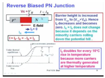
Make this side; right side more positive compared to the negative side, how do I do that? I apply voltage across the junction with this N side more positive compared to the P side, so that is like this. So, I made P side +, I applied a still voltage VC which you can call it as VR, you call it as a reverse bias. You call it reverse bias because you have increased what if originally the height was VCP or VBI, now you applied both this side.
