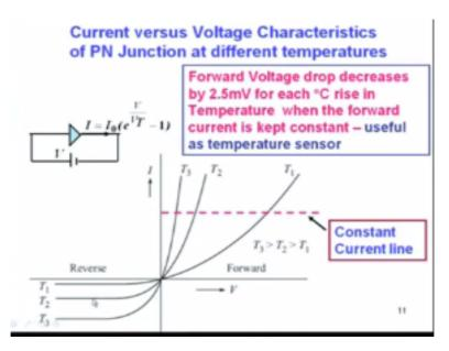
So, now the IV characteristics, forward bias I = I0, e to the power VE/VT -1 that is the characteristics at room temperature t1 exponentially increasing and forward bias, reverse bias; reverse is polarity, V is negative, so e to the power – VE/VT; VT is about 25 electron volts, VT is actually KT/q, K is Boltzmann constant, T is temperature, q is electronic charge.
