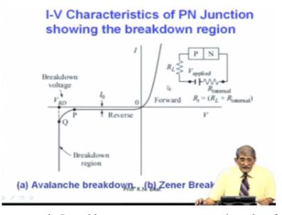
In the sense, you can use it, I would access or temperature sensing when forward bias was kept constant, you can measure the voltage doubler thing, as a function of temperature, so you can calibrate it by noting that the forward voltage drops by 25 millivolts for each rise, degree centigrade rise in temperature. So, this is actually the full characteristics, forward characteristics, reverse characteristics, this is I0, e to the power VE/VT.
