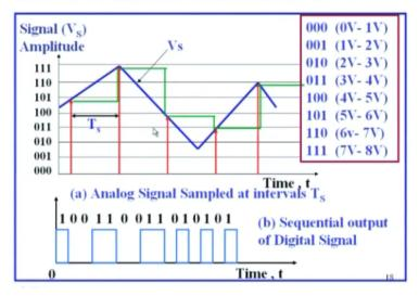
Illustration of A to D Conversion in a 3-bit ADC
