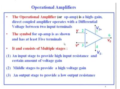
Let us take a look at this operational amplifier. This is a very popular device. Operational amplified is a high gain direct coupled amplifier, which operates with the differential voltage between 2 input terminals. Whatever is the difference voltage, it gets amplified. If there is a common voltage, then a difference voltage 0 at that point, if you apply even the voltage between the 2 same, output will ideally be = 0.
