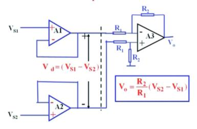
Now you can choose the different that you are opting noise, I do not want that very high gain. Because if I am getting already very high gain by means of this R2/R1, I had want only a fixed gain. I can change this. In this case, I can change the gain by changing Rg, but if I remove this Rg, then use it like this. I remove the Rg, use this as unity gain amplifier, whatever you get here the Vd here is Vs1-Vs2. How is that possible. Vs1 is same as here Vs1.
