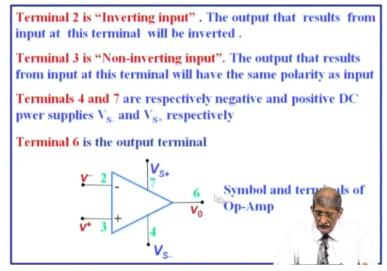
There are several terminals. The ideal one or the most important terminals are, I have marked it as 2, 3, 4, 6 and 7. 1, 5, etc or other terminals, which I am not showing. Terminal 2 is inverting input. The output that results from the input at this point will be of offset polarity. For example, if I have +1, there will be -1 here. Terminal 3 is non-inverting input, the output that results from this has same polarity. If I apply +1 here, it + voltage here with an amplification.
