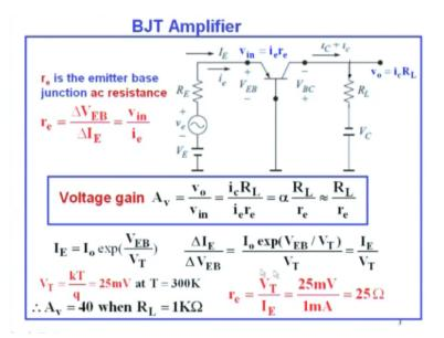
So we saw last time. I just had quickly gone through this portion of BJT common base amplifier circuit. Here, what I would like to point out is there is DC as well as AC. The DCVE is connected to the emitter lead through a resistance RE so that the emitted current is fixed by this loop = VE divided by RE approximately. Strictly speaking it is VE – VEB divided by RE, but VE will be large compared to VEB, because VEB is the order of 0.65 volts.
