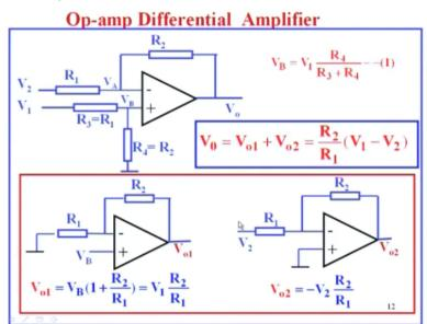
Now let us take a look at differential amplifier using an op-amp. Here you can see that V1 is applied to the non-inverting terminal to this resistor and V2 is applied through this inverting terminal to the output like that. So what we want to find is what will be the output voltage for this case. V1 and V2 are applied. You can analyze this very simply by considering this circuit as superposition of these two circuits.
