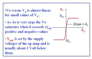
**Op-amp transfer Characteristics (V<sub>o</sub> versus V<sub>d</sub>)**
