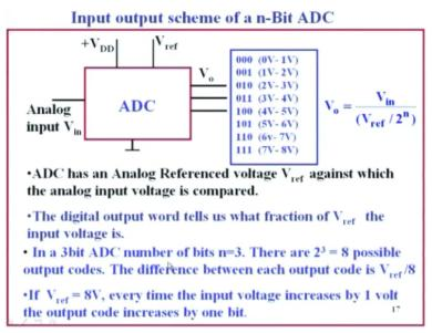
So the input output scheme of a n-bit ADC, now for example, what is the being of n-bit. If there are 3 pulses to decide 1 word, then this is called 3-bit. For example, I can write a number, a voltage 0 as 000. There are 3-bits are used, each one is a 1 pulse, here all the pulse are 0. Second one, if you take 001 pulse is 0, pulse is 0, third pulse is 1 that is high, the pulse is present here. Now in a digital form 001 is 1 so it may represent 1 volt, 010 in a digital form is 2, 011 is.
