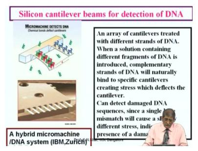
Now leaving the topic of pressure sensor and the system resisted that, just see that this is the silicon. We will take a look at this silicon cantilever beams for some DNA detection. Here, you have got an array of cantilever anchored here and this will get deflected whenever a molecule or DNA strand comes and rests on that. So here the trick is to dip this in a solution containing different fragments of DNA.
