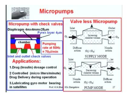
Now, this is the micro pump which we have discussed just now, and in that particular system that I have shown the flow rate is, pumping rate is 70 micro litres per minute for that dimension. How much is the flow rate would depend upon, what is the frequency of the voltage that we are applying. One stroke you will have small quantity of flowing. In one minute, how many cycles are there, it is 50 hertz, 50 cycles, you have 70 micro litres flowing.
