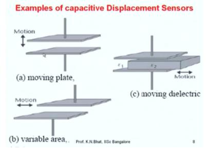
Now what you need to do is, you have to measure the displacement of the mass. Going back to previous slide, what you want to measure is how much is the displacement x for a given force. So if I measure the displacement x, knowing this mass and the spring constant, I can find out what is acceleration, what force is. So the entire theme of accelerometer is based on measuring the displacement. There are several ways of doing that.
