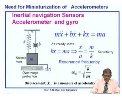
The next one, I am just touching upon these miniaturized accelerometers. A quick look at that, you would have discussed it already, but you know that this is an accelerometer system, is a combination of a spring and a mass and the mass is attached the spring. The spring is anchored to the body from air. So if the mass experiences a force, it will get elongated. It will be going down in that direction if you force in that direction.
