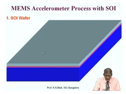
The way it is made you can just quickly see that this started this silicon, the entire thing is silicone, top is silicon, red is oxide, this is silicone. Now by means of a technique of photolithography, you can pattern this top layer, etch silicon from the regions where you do not want the silicon that. You can see that previous slide you had this color everywhere, now we have removed the silicon from everywhere else except in these portions.
