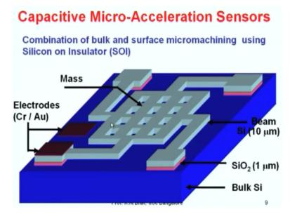
So find out the change in capacitance to determine the displacement and ultimately the force or the acceleration. Now, this is structure of a micromachined accelerometer. Here, this particular region, the central one with holes is the mass. The hole is provided to adjust the damping between the mass and this bottom plate. So when it moves, if there are a sufficient number of holes, the squeezed film damping can be adjusted by adjusting the number of holes.
