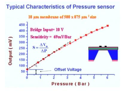
Here on the y axis here are the output in millivolts and on the x axis you have the pressure that the membrane is subjected to in the case of intracranial pressure monitoring, it is the intracranial pressure experienced inside the brain or on the brain. For a 10 micron membrane of this dimension, 500 micron by 875 micrometer square, you will get a voltages of several millivolts. Ideally, you do not need any electronics. You can as well use these output voltage.
