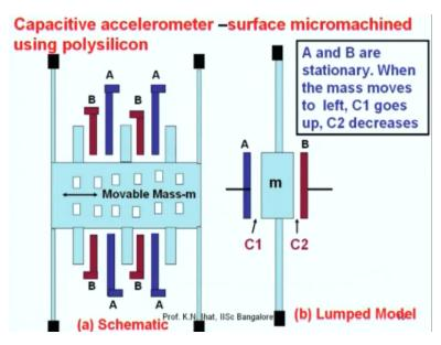
Now these are variations of that. I will have occasion to discuss this later. The previous one was the 2 electrodes, which are on both sides of the mass and the mass are moving only in the vertical direction. Now this is actually a mass, which is anchored in these 4 portions. The rest of the thing is able to move in this direction, in the horizontal direction, like that and these are the fixed electrodes and each electrode marked A is connected together to form one electrode.
