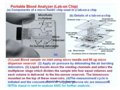
Now the other one that I want to mention here is the blood analyzer. This is a very classical example of a microsystem, which is also called as the lab on chip. The lab on chip here is not very clear there are multiple things. One is if you break it up in to subsections, you can see there is a region where you can inject blood sample via this inlet using microneedle and fill up the micro distance here, the reservoir. So how do fill up these small quantities of blood.
