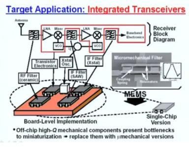
Now do not get frightened, this is actually the trans receiver in your mobile. All these within that is electronics and in addition to electronics, all these are filters, ceramic filter, then voltage control oscillators, saw filters. These all take a lot of space. So the goal is to change these filters with small size mechanical resonator so that the entire thing can be made. Where this entire electronics can be put in a single package. It is very small.
