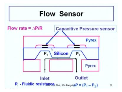
Now the other one, there are 3 components, I mentioned. One is the mixture where different channels will come and merge. The other one is flow sensor in each of those channels. You can just understand this flow sensor from the principle of flows like a current in electric circuit. If you know, if you have a resistor, if I apply voltage across the resistor, the current through the resistor will be voltage by resistance.
