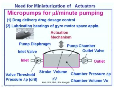
This is a micro pump. So you will have several micro pumps going through the channel, and the flow sensor and through the mixture and the principle of that is a chamber and a membrane, which can deflect and moved up and down and a inlet valve and a outlet valve. The valve will open only in this direction, inlet. This valve will open only in that direction, outlet. This is the size of the pump on a thumb, that is what we are talking of, for bio-medical application, space applications.
