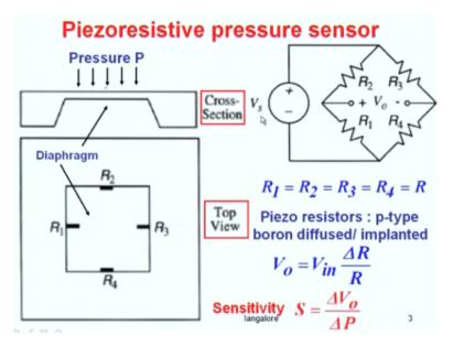
This is actually inside the package. What you will have will be a membrane as shown here, which in this case in a microfabricated pressure sensor, it will be a silicon membrane. The thickness of the membrane may be 10 microns, 15 microns, or 20 depending upon what pressure you are monitoring, lower the pressure, thinner should be the membrane, so that the sensitivity is better. So this pressure is experienced by this membrane and that stress actually gets amplified over the edges.
