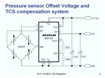
You use this bridge, the pressure sensor along with a chip, you can use for example Maxim, Max 1452 is a very popular chip that is used along with this. You can have it mounted along inside the package. You can have this pressure sensor as well as this chip that is put together in the package and that is the microsystem. Alternately, you can have the entire circuitry decided along with this particular resistor on the silicon itself. That is fully integrated.
