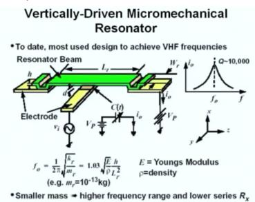
Now the last of the thing I want to discuss today is the filter. When you say filter, it is an electrical filter. If you see a signal passing circuit like the transreceiver. If you take your mobile, it is able to transmit signal, it is able to receive the signal and they are all at high frequencies, modulated signals. You must get from that high frequency, the voice signal. So you need to filter out some of the high frequencies, you need to convert that entire signal back into voice.
