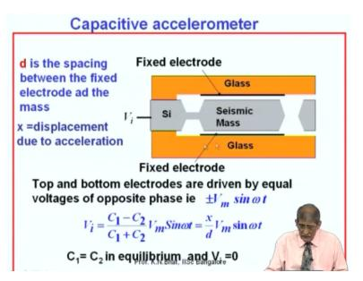
So what you do is, instead of using one plate like that use a mass, which is called as Seismic mass. Seismic is referring to earthquake. So these mass can be used in this type of accelerometer, can be used to sense even the very small low frequencies, which are seen or experienced during the earthquake. So this is the mass, which is anchored here. This is a glass. It is different from the previous accelerometer, which I showed. So this is the mass, which can move up and down.
