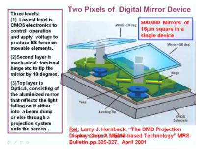
This is another system, digital micro mirror devices, which has, this is a very classical example of a micro system, which has lowest level. 3 levels are there. Lowest level is the CMOS electronics to control the operation and apply voltage to produce electrostatic force on the
