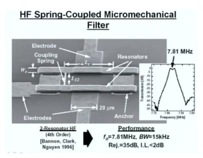
One beam, another beam, there is a mechanical connection between the 2. They will be moving, trying to move together. Each one will be pulling together with respect to other frequency, so which is the one frequency, you will get a band of frequencies that is called band pass filter. So use this band pass filters in all your trans receivers.
