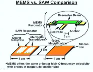
But the entire thing can be taken care of by one beam like that, which is like that. So what is 1 cm by 1 cm can go in by a few micron size here. So going back to the previous slide, this entire thing, the goal is to replace the entire thing by means of one such structure like this. you can have many more of them to represent different frequencies that are size can be reduced and quality factor will be excellent provided the whole thing is put inside a vacuum.
