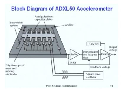
This is the block diagram of the ADXL50 accelerometer of analog devices, which is used for releasing or deploying the airbag in a car. You can see that this is the mass, which moves. These are the fixed electrodes and both are connected together to ensure that it can measure the capacitance between one electrode and the other, between the 2 you can do in this electronics. We will come back to this later.
