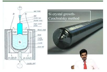
The fabrication of silicon wafer although we hardly follow those in university lab, you almost always buy the silicon wafer from the vendors but still it is interesting to see how you can get that silicon wafer out of silicon.
