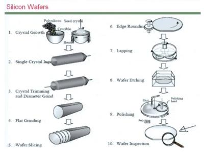
So we you know have a series of process steps essentially you know fallout to build a single crystal which is fashioned you almost like a cylinder, and essentially run through a series of steps further to final year result in a completely flat wafer. So it is essentially by melting the silicon or which is essentially a high purity sand that you get silicon as a source material, and it is absolutely critical that at this stage itself the crystal orientation of the silicon is defined.
