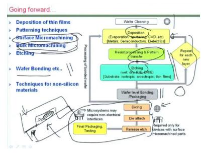
So going forward in the subsequent lectures what we will see is that how silicon and other substrate materials that you have seen could be started with and how some of these process steps could be done to build really what are called this moving components and you know so that we can build microsystems. Let me give you a brief overview of how these are done.
