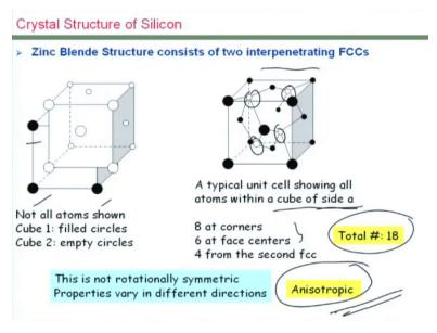
Now why is it that we have all these different types of wafers and what makes difference as I mentioned in the case of silicon is essentially a zinc-blende structure which is consisting of 2 cubic lattices which are essentially interpenetrating FCCs. So in the example in the schematic here the 3 atoms from one of the cubic is marked with this black darkened circles and some of the atoms from the second interpenetrating FCC are marked with this hollow circles over here.
