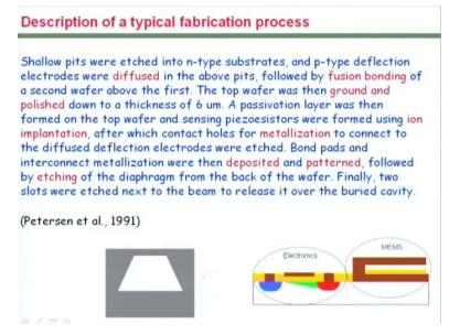
Now let us look at you know how the processes are arrange, which are the process that could be required in building a typical microsystem, what you see here is one of the oldest example of building reported for building a micro system in this particular case a pressure sensor. And if you read through the passage over here what we have is that if you see coloured is that a series of process steps many of these are you know are used in IC fabrication as such.
