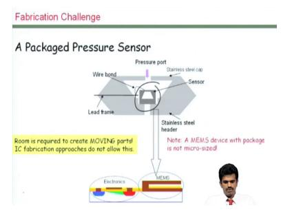
One example another common example is pressure sensor, which essentially has a small chip in the middle which is actually you know package by this extra enclosure, so that you know the interface is possible and what is inside there could be you know based on the fabrication technologies that I have I will just talk during this lectures.
