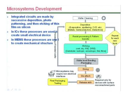
Now for the microsystems development the flow that you follow is quite similar to what is done in IC fabrication. We start with clean wafer and do a series of steps such as deposition and patterning which are done repeatedly and then we do some sometimes we do wafer bonding and we also and that again can be followed multiple times, and ultimately after all these are done we dice them into individual chips and then attached the package and then package will do that.
