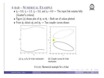
Let us look at an example. So, we have  $l_0 = 5.0$  so, the base link is chosen as 5,  $l_1 = 1.0$ ,  $l_2 = 3.0$  and  $l_3 = 4.0$  arbitrarily chosen but chosen with the goal that the input link will
