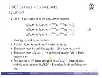
Again we use the S-S pair constraint. So, between the first contact point and the second contact point, these are modeled as an S-S pair. So, the distance between that must be constant. So, between  $p_1$  and  $p_2$  ok, the distance is  $k_1^2$  very similar to what we did for the 3 RPS case. So, this equation will contain  $\theta_1$ ,  $\psi_1$ ,  $\phi_1$ ,  $\theta_2$ ,  $\psi_2$  and  $\phi_2$ .
