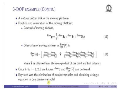
The problem is not yet finished. We need to find the position and orientation of the output link or the end effector. So, in this case, the natural output link is the moving platform, the top moving platform. The position and orientation of the top moving platform, we can assume that the position is the centroid of the top moving platform, which is nothing, but the sum of the vectors connecting the three points on the top platform.
