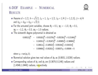
So, let us do a numerical example. We assume  $;d = 1/2, h = \sqrt{3}/2$  and the actuated joint variables are arbitrarily chosen as 1, 1/2, 1/4 and so on and then, this distance between spherical joints are assumed to be equal to  $\sqrt{3}/2$ . So, for the chosen actuated joint variables  $\theta_1, \psi_1, \theta_2$  and  $\psi_2$  all in radians ok.
