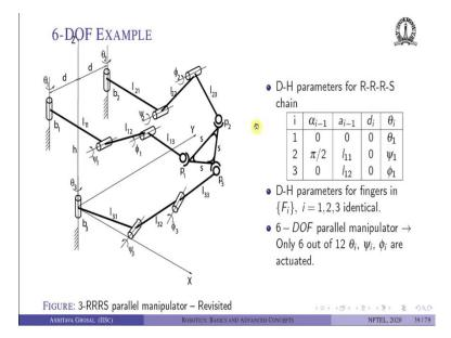
So, let us continue. Hence, look at another example which is the 6-degree of freedom example. So, this as I have mentioned earlier, it models a three fingered hand gripping an object. So, these are the three fingers  $b_1$  which is fixed base  $b_1$ , then  $l_{11}$ ,  $l_{12}$ ,  $l_{13}$  these are the finger elements or the link lengths in the finger and likewise, we have another finger, and we have another finger third finger ok.
