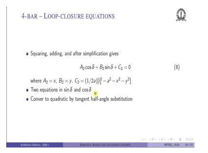
And again, square and add these two equations, we will get another equation in cos and sin  $\delta$  ok. So, it will be  $(A_2 \cos \delta + B_2 \sin \delta + C_2 = 0)$  and again,  $A_2$ ,  $B_2$ ,  $C_2$  are quantities where  $x, y, l_1, a$  and so on other quantities appear. There are no angles again in  $A_2, B_2$  and  $C_2$ . So, we have two equations in sin  $\delta$  and cos  $\delta$ .
