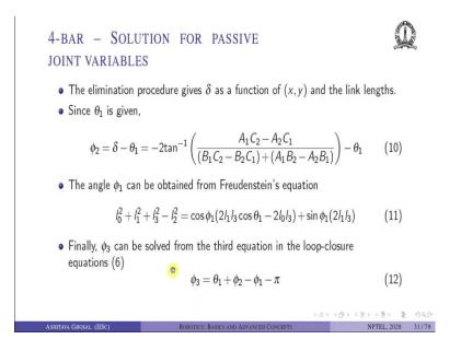
We can also continue, and we showed you that the elimination procedure gives  $\delta$  as a function of *x*, *y* and the link lengths. We can also find out the joint angles. So, given since  $\theta_1$  is given, we can find out  $\phi_2$  which is  $(\delta - \theta_1)$  and
