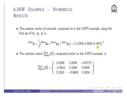
So, as we see in the direct kinematics, we now need to find the position and orientation of the moving platform which is the chosen output link. So, again we will assume that the <sup>Base</sup>p which is the centroid of the top platform is given  $(1/3)({}^{Base}p_1 + {}^{Base}p_2 + {}^{Base}p_3)$  and we will get an X, Y, Z coordinate of this form. So, X = 1.37 so on, Y = 0.261 and Z = 0.1401.
