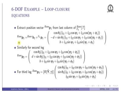
So, we multiply all this four this how many are there? So one, two, three, four and five transformation matrices and then, we extract the position vector of the last link last transformation matrix, the resultant transformation matrix. So, this will give the position vector of the spherical joint 1 with respect to the  $\{Base\}$ .
