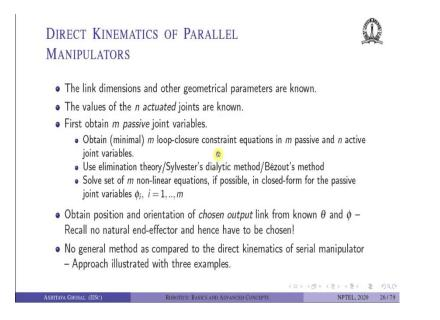
So, in the direct kinematics of parallel manipulators, the link dimensions and other geometrical parameters are known. The values of the n actuated joints are known. So, remember in the parallel robot as discussed in the last lecture, there will be some n actuated joints and m passive joints.
