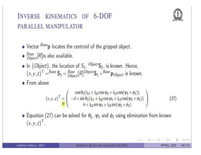
So, how do we do this? It is not very hard because we have just the position vector of a point which is let us say the centroid of the gripped object. The rotation matrix of the object with respect to base is also given.
