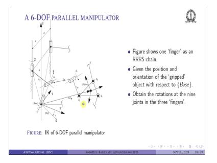
Let us look at a 6 degree of freedom parallel manipulator. So, in this case we have looked at this 3 fingered hand ripping an object. So, I am showing one finger as an R-R-R-S chain ok. So, the other two fingers are not shown. So, what is given? The position and orientation of the gripped object ok.
