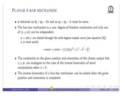
Again  $\phi_1$  obtained as  $(\theta_1 + \phi_2 - 2\pi)$  and  $(\phi_1 + \phi_3 - \pi)$  must be same ok, if you think about it. Whether you obtain from this side or from the other side both must be same. The 4 bar mechanism is a one degree of freedom mechanism and only one x, y or  $\phi$  can be independent ok. So, we need to make sure that the x and y are related through the sixth degree coupler curve and  $\phi$  must satisfy  $(x \cos \phi + y \sin \phi)$  is given by this ok.
