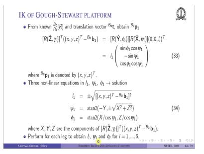
So, that is what is given here. So, this x, y, z which we have obtained from the coordinate of the S joint minus  ${}^{B_0}\boldsymbol{b}_i$ , will give a vector along this length ok. So, that is what is given as some rotation matrix because we need to multiply this vector and this is given as first one rotation about a the U joint another rotation that the U joint and a translation along the length ok.
