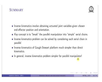
In summary the inverse kinematic involves obtaining actuated joint variables given chosen end effector position and orientation. Again the key concept is to break the parallel manipulator into simple serial chains.
