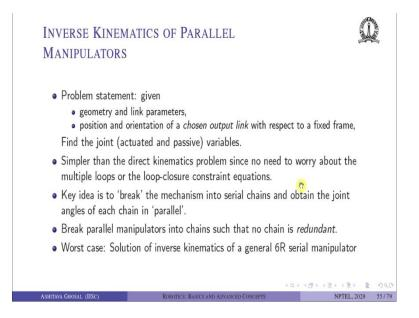
So, what is the problem statement in inverse kinematics of parallel manipulators? We are given the geometry and the link parameters and the position and orientation of a chosen output link with respect to a fixed frame and the problem is to find the joint variables. Now, in this case we have both actuated and passive joint variables.
