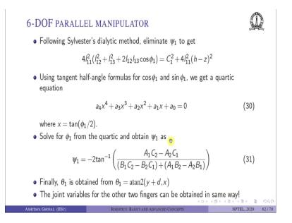
And then we use the Sylvester's dialytic method, which eliminate  $\psi_1$  and we find out the determinant of Sylvester's matrix equal to 0. So, in this case that will lead to this equation, one single equation in  $\phi_1$  equal to all this constraints. So,  $C_1$ ,  $l_{11}$ , z, h all these will show up ok.
