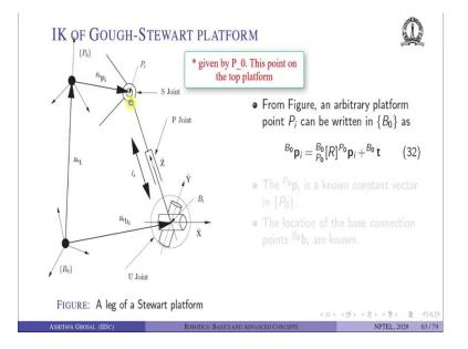
Let us look at this inverse kinematics of the Stewart-Gough platform this is a very famous platform 6 degrees of freedom Stewart platform. So, what do we have here? We are looking at one leg of the Stewart-Gough platform. So, there is a fixed coordinate system  $\{B_0\}$ . There is a coordinate system which is attached to the top platform which is given by  $\{P_0\}$ . This point on the top platform which is an S joint is located by this vector  ${}^{P_0}\mathbf{p}_i$ .
