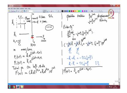
So, this here is my unbounded partition goes off to infinity in two directions up and down this is my x axis over here and the partition has a mass m per unit area it is mounted on springs, the spring stiffness is also s per unit area and mounted on viscous dampers which are also r units per unit area and the left side has medium properties  $\rho_1 c_1$  density  $\rho_1$ , speed of sound  $c_1$ and right side has  $\rho_2 c_2$ .
