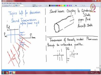
Which is transmission, transmission of normally incident plane waves through an unbounded partition. So, there is an unbounded partition which goes off to infinity up and down and there is a plane sound wave incident on it, there is a plane wave incident on it, and this is mounted on some springs and dampers and so forth and we want to find out what is transmitted to their site? So, let me draw the geometry properly.
