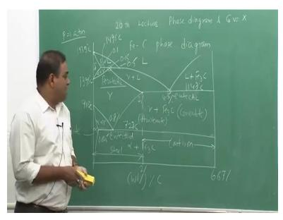
Now this iron carbon phase diagram would be very critical mostly the solid this steel part you we have two parts, one is steel part one is cast iron part. The steel part would be very critical because we will be looking at heat treatment of steel in the steel part only, okay though of course you can have lot of other heat treatments available for the cast iron part. So we will be concentrating on the steel part.
