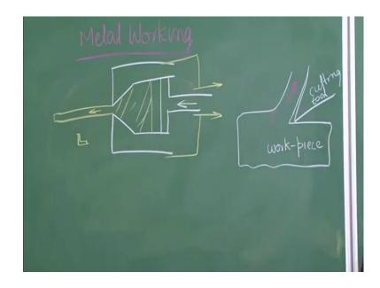
You have a die like this and inside you have a piston which moves like this and in here, you have metal which is forced through this orifice and you get longitudinal structure. Now this longitudinal structure can be of any cross section, for example, it can be a I section, you remember you having seen those L frames, the aluminium shaped L frames, this is how their manufactured.
