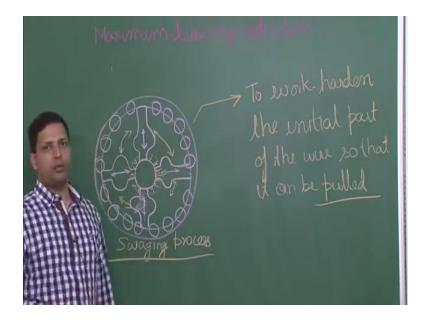
But anyhow at some point it may break and in that case you will have to have to do this work hardening, how it is done? So it is a swaging is a process like this let us see this is the final diameter that you want it will have a hammer kind of structure. So, these are four hammers which can move in and out like this and there is a fourth one over here. So, what next one goes in and out? There are spherical balls all around, so these spherical balls are still inside another cylindrical structure.
