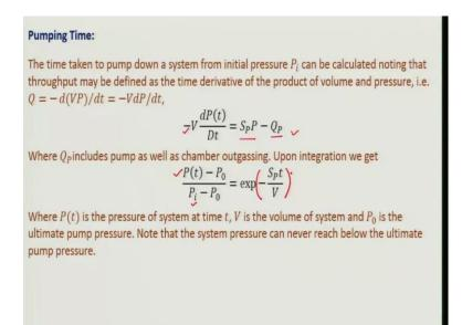
Now, suppose you have chamber which you have connected through some pipes to a vacuum pump and you have some leakage also how much time, it will take to pump it down to a certain level. So, as we had seen, this is change in pressure, pressure is going down that is why we have used negative sign volume is constant DP by DT is the throughput of the pump and this is the throughput of vacuum pump minus leakage if you
