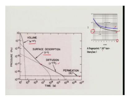
How does vacuum process works with time? Remember when we have looked at the pumping time, we have said this has exponential relation with time, some kind of exponential relation this is called volume pumping. So, in this stage you are taking out the volume of the gas.
