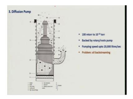
The third type of pump is diffusion pump and the diffusion pump can go up to 10 to power minus 10 Torr, it is backed by rotary or roots pump for the similar reasons that we do not want the initial our good pumps to handle the bulk of the gases. So, first we want to remove the bulk of the gases or which may have some particle metal dust etcetera by roots or rotary pump than we pump switch on the diffusion pump so that the load on this diffusion pump is less.
