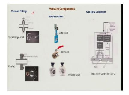
They are different type of vacuum fittings, quick flange or conflate vacuum valves where you can control the pressure by other nomadically or computer controlled or manually or you can close a valve or open a valve or also sometimes when you have to flow a gas into the system a pure gas then you can use of mass flow controller to introduce the gas at a control trite. These are all part of the vacuum system.
