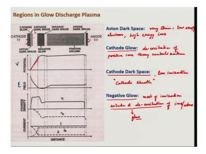
Now, if you have a plasma between 2 electrodes, they are different regions of the plasma, it is not uniformly distributed, what are these different regions are shown in this curve; in this diagram on the top and how the potential field v, electric field, charge density, number of ions and electrons and the current there is in these different regions, it is shown below this diagram, we will discuss few of these regions which are of most important to us.
