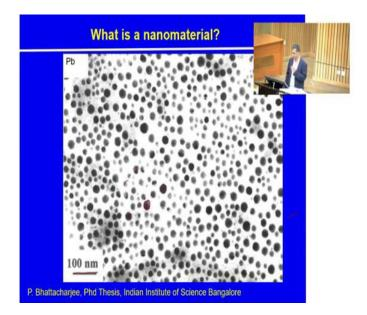
So, first of all about the recap you know what is the nanomaterial? And, in the last lecture I showed you this particular image. This is basically image obtained for lead nano-particles using transmission electron microscope. What is the transmission electron microscope and how does it operate? We are going to discuss about it later when we talk about characterization. For the time being we focus on the image.
