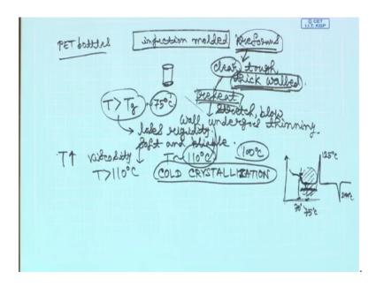
So, basically when you are creating the PET bottles how do you do that? So, first you start with what you call I will come to this process after injection molded preforms you start with. So, injection molding is a process through which you can prepare different kinds of shapes of the material. So, you start with what you call as a preform a small structure.
