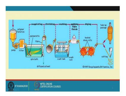
So, you are starting with a polymer solution and then you are push pushing it through a filter of course, because it has to remove all the foreign particles so on and so forth and whatnot now and then you are pushing it twist through a what it looks like you know your shower head, which is your spinneret basically. This spinneret is dipped in a in a bath of liquid and this liquid is miscible with the solvent used to make the polymer solution, but the polymer itself is not soluble in this liquid.
