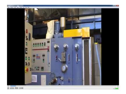
So, the first video will be the video of the polymer melt spinning. So, you see this is your this is in general how it looks the machine, polymer pelletes that were pushing fitting here this is your starting material and then your full process is automated.
