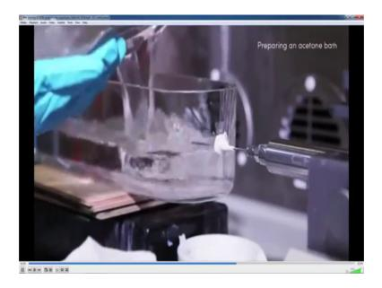
So, you see this is an acetone bath being prepared because the polymer is not soluble in acetone and then when you are pushing it through basically it is in water suspension. So, water is miscible with acetone, but nano cellulose just comes out because it is not miscible with acetone and then you can just drag out these fibers like this. So, you have all these fibers that has been produced and you can dry them up by suspending them like this in the air.
