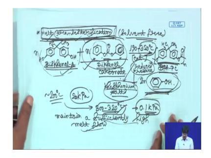
So, one of them is melt transesterification. So, basically this is a solvent free process and as the name suggests this is transesterification. So, again you start with a Bisphenol A this in this case you are not using a Bisphenolate salt because you are not using a solvent in which it has to be dissolved. So, you can just use the parent Bisphenol A
