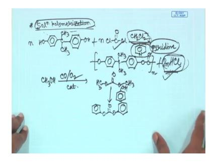
The third process through which you can prepare polycarbonate is solution polymerization basically this is very similar to your interfacial polycondensation, but here you are not using two solvents you are basically using only one solvent which is your organic solvent. So, it is done in one phase not like in two phase.
