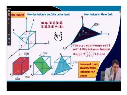
So, when we understand the atomic positions of the cubic and the hexagonal unit cell. Let us start with understanding the Miller indices of these unit cells. Let us start with the cubic structure and we will only show the cubic structure and I hope that you will go home and learn the Miller indices of the hexagonal close-packed crystal and I hope that most of the students who are doing this course may have already know the what is Miller indices and how it is found out.
