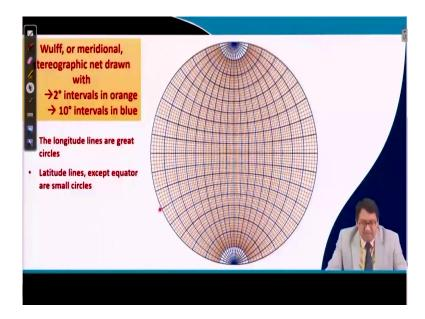
So basically a Wulff net which is basically cooler to observe and quantify the stereographic projection is shown the orange-colored Wulff net has basically degree graduation of 2 degrees and the blue colored Wulff net has a graduation of 10 degrees.
