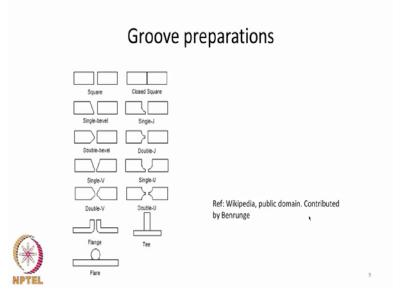
So how detailed can the joint preparation or edge preparation be in a groove weld is clear from this set of groove preparations. The image has been taken from a Wikipedia, but these joints are name are used in the literature quite commonly; so we have what are called square, closed square, single-bevel, single-J, double-bevel, double-J, single-V, single-U, double-V, double-U etcetera.
