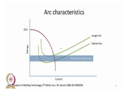
So, there are some characteristics of the arc that we need to be familiar with so that we can understand why the voltage and current condensations that are chosen for welding are like that. So we are seeing in this a plot, a red curve that is going from top to bottom, and this curve is also called as the drooping characteristic of the power source.
