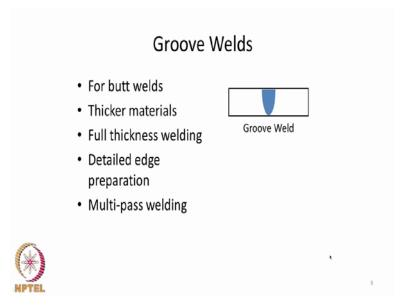
Groove welds are once that are used for large thickness joints. So these are also usually made in butt geometry and the large thickness also implies that we will have the weld penetrating to the entire thickness, and that would require a very detailed edge preparation. And very often the welding techniques may not be able to join the entire thickness in one go, so we may have to resort to what is called as a multi-pass welding.
