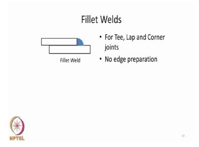
Fillet welds are `what are used to join materials when they are kept in lap geometry. And tee, lap and corner all three can be joined in this mode of fillets welds. The advantage of this particular way of joining is that there is no edge preparation; however, there is a requirement that you need to have filler.
