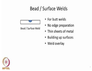
Little bit details about these; a bead or a surface weld is used very often for a butt welds; and the advantage of this geometry is that there is no edge preparation that is required; and this is used for thin sheets of metal. And this is also used for example, to build up surfaces. So if you want to repair a part, then you can remove some material by gauging or any other metal removal process and then the material can be build up at the same location again by making a bead on top of material.
