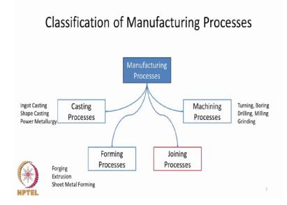
Let us first look at under what over view does the joining on welding processes come under. We have basically a large number of manufacturing processes, which can be categorized broadly as casting processes, which are the primary manufacturing processes, such as ingot casting, shape casting, powder metallurgy etcetera. And then forming processes, where we a change the shape by using processes such as forging, extrusion, deep drawing, sheet metal forming etcetera.
