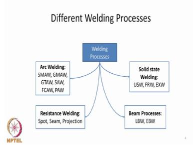
And welding processes again can be categorized by a different source of joining. The first set is by arc welding, where there is an electric arc that is used to join the two materials. I have given the acronyms here as per the AWS - American Welding Society specification.
