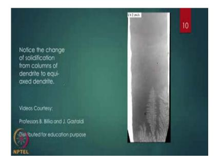
In this video, what we are actually going to show you is a transition from a columnar to equi-axed microstructure formation. We have already seen that as we increase the solute undercooling this kind of a transition will happen. At the top, you see that the velocity is going to be changed; and when the velocity changes to a higher value, you would see what is happening. And let me play the video for you. This is initially a dendritic growth,
