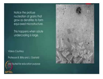
So, we can look at the equi-axed mode again a bit closer in a smaller domain by enlarging it. And you can see that essentially what is happening is that in the liquid, these dendrites are being nucleated and then they are growing up to a particular extent, and then settling down; and each of these dendrites may become one grain. And because they are growing roughly equal in all directions you see them as equi-axed.
