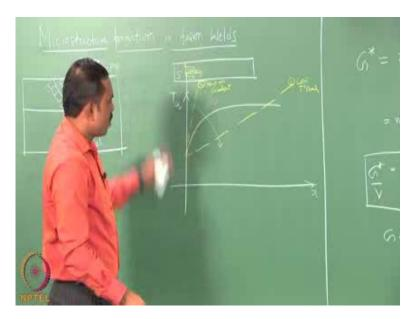
Now, this would actually allow us to make what is called as a map the map of how the solidification is happening; and that map would tell us overall the picture of how the microstructure will be in the fusion zone. Before we make the map, you just look at the situation step by step as we go from the temperature gradient at a high value to a low value as we keep decrease in the temperature gradient what is happening.
