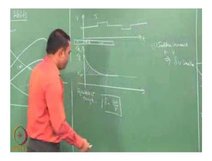
We can also analyze it to see what would happen using a small schematic. So, the way we analyze the schematic is as follows. Let us say as a function of time, the growth rate is supposed to be kept constant, but for whatever it has not been kept constant. And let us say it took a high value and then came back to the same value. And then after sometime, we took a low value and came back to the same value.
