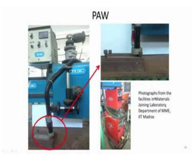
And here is a setup that shows how a plasma arc welding setup would look like from our materials joining laboratory in Department of MME - IIT, Madras. And you could see that the torch assembly is little bit more involved compared to a TIG welding torch, and then the torch is then mounted on a drive that could make the torch move along a path at a given velocity.
