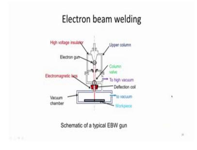
The last two processes which are basically high power beam processes or electron beam welding, and laser beam welding. So electron beam welding process is shown here as a schematic.
