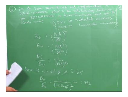
So we will move on to the problem six. So the question is for the same value of numerical aperture and magnification in an optical microscope what is the relationship between the brightest in trans illuminator and epi-illuminator mode. So we have seen these two types of eliminators in optical microscope; we can write for our clarification. So epi-illuminator is generally reflected mode and trans: transmitted transmission microscope.
