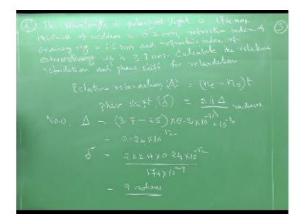
We will now see the next problem that is fourth problem. So the problem here is the wavelength of polarized light is about 174 nanometers, thickness of the medium is 0.2mm, refractive index of ordinary ray is 2.5 nanometers, and refractive index of extraordinary ray is 3.7 nanometer. Calculate the relative retardation and phase shift for retardation see the retardation and the phase shift we have looked at in the fundamentals of light optics.
