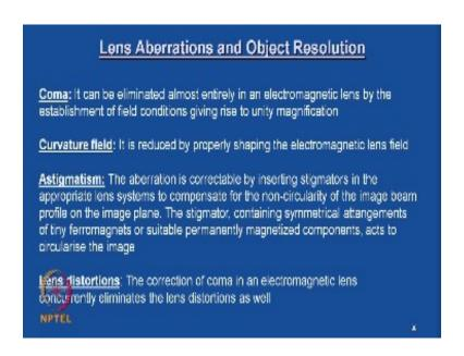
In terms of coma it can be eliminated almost entirely in electromagnetic lens by the establishment of field conditions giving rise to unity magnification and in terms of curvature field it is reduced by properly shaping the electromagnetic lens field. The astigmatism on the other hand is correctable by inserting stigmators in the appropriate lens system to compensate the non-circularity of the image beam profile on the image plane.
