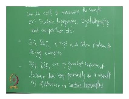
And also the crystallography of the specimen and that under its chemistry can be analyzed with the scanning electron microscope primarily. So, what what, what are the parameters which enables this microscopy to do that. We will see that. So, what are the typical signals we are going to get from the SEM, secondary electrons, backscattered electrons, x-rays and other photons of varying energies.
