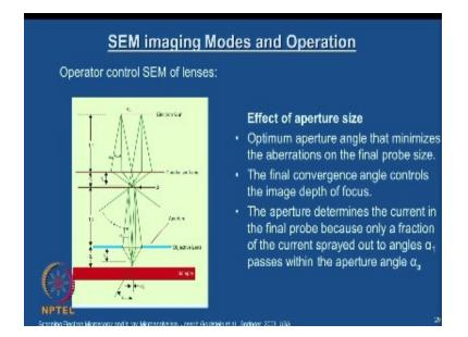
We will just quickly review this. We just started looking at the operator control in SEM of lenses. We have three primary parameters. One of them is the aperture. So, this schematic clearly shows that if the final aperture which basically controls the probe diameter which finally impinge on the sample the bite controlling this objective lens and this is what we just summarized here the optimum aperture angle that minimizes the aberration on the final probe size.
