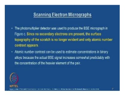
The photomultiplier detector was used to produce BSE micrograph in Figure-C. What we have just seen in two slides before, since no second electrons are present the surface topography of the scratch is no longer evident and only an atomic number contrast appears. Atomic number contrast can be used to estimate the concentrations in binary alloys because the actual BSE signal increases somewhat predictably with the concentration of the heavier element of the pair.
