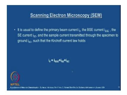
So, now we will look at the much more detail about this the probing current and so on. It is useful to define the primary beam current  $i_0$ , the backscattered electron current  $i_{BSE}$  the SE current is  $i_{SE}$  and the sample current transmitted through the specimen to the ground is  $i_{SC}$  such that the Krichoff current law holds so the primary bream current can be s can be represented as
