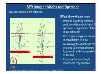
We also define this what is the working distance. It is the distance between the final aperture and the specimen surface and you can clearly see this effect of working distance from these two schematics which is quite evident that, if you increase the working distance you are increasing the probe size. You carefully look at it. You can see that the probe size is increase now and obviously it will have some significant effect on the resolution.
