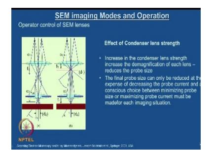
So, the final probe size can only be reduced at the expense of decreasing the probe current and a conscious choice between minimizing the probe size or maximizing the probe current must be made for each imaging situation. So, this is exactly I was just mentioning that, all these parameter controls has to be done as per the requirement for the appropriate information we are looking at from the specimen and it is completely in the user control.
