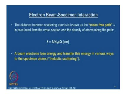
The distance between scattering events is known as the mean free path lambda ( $\lambda$ ) is calculated from the cross-section and the density of the atoms along the path.
