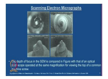
The another important aspect of this SEM be mentioned is a depth of focus and this set of micrograph clearly illustrate that aspect. So, what you see here is, a, this is a machine screw viewed at under the optical microscope and this is understanding electron microscope. You can see that in an optical microscope, you do not see any of this detail when you look at this crew from the top. You can see the all the other the circular details of the screw and C and D are taken
