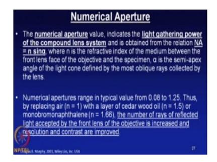
This numerical aperture range in the typical value from 0.08 to 1.25. Suppose this is for this is for the medium air where the refractive in the index is equal to 1. Suppose if you replace this with the layer of cedar wood oil which has got the refractive index of 1.5 or mono bromo naphthalene which has got a refractive index of 1.66 the number of rays of the reflected light accepted by the front lines of the objective is increased, and the resolution and the contrast are improved.
