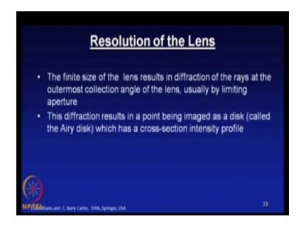
Let us look at this before we see the animation let us look at two more points the finite size of the lens results in the diffraction of the rays. At the outermost collection angle of the lens usually by the limiting aperture. This diffraction results in your point being image as a disk called the airy disk. This has the cross-section intensity profile.
