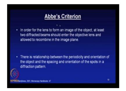
It is Abbe's criterion, in order for the lens to form an image of the object at least two diffracted beam should enter the objective lens and allowed to recombine in the image plane. So if you go back and see the image animation what we what I showed in the last class it is very much clear that the rays which is coming from this periodic object the orifice from O1, O2, O3.
