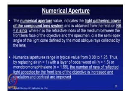
Now we will move on to the other important parameter called numerical aperture. We have seen that in the very definition of the resolution : this d equal to the inversely proportional to this numerical aperture that is what we have seen so in order to understand this what is the numerical aperture first we will just look at the introduction remarks the numerical aperture value indicates the light-gathering power of the compound lens system.
