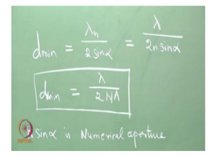
So now you will appreciate the resolution definition we just stated before we get from this a path difference ray diagram a small derivation and then now we will see the effect of the numerical aperture on the resolution we can simply write either increase in numerical aperture that means the light collection ability of the objective lens increases or decrease in  $\lambda$  will produce the same
