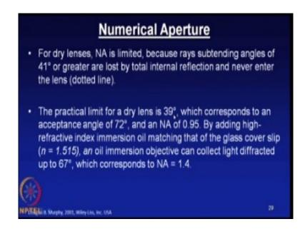
Let us look at a few more points on the numerical aperture, so whatever I just stated before : for dry lenses numerical aperture is limited because, the Rays subtending angles of 41°.
