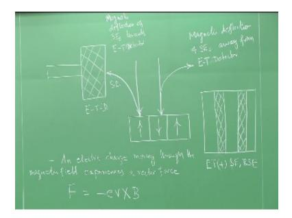
So, you see a schematic which I have drawn here is, this is an ET detector and this is the specimen we talked about. And there are two distinct events happen here. Because of this an electric charge moving through the magnetic fields expresses a vector force
