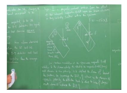
So, this type 2 contrast or magnetic contrast arises from the effect of internal magnetic field upon the beam electrons as they initial scatter within the specimen. So, it is the interaction between the internal magnetic field and the beam of electrons after they initially scatter within this specimen. I need to draw one schematic again based we will use the same equation here also F=-vxB so you have.
