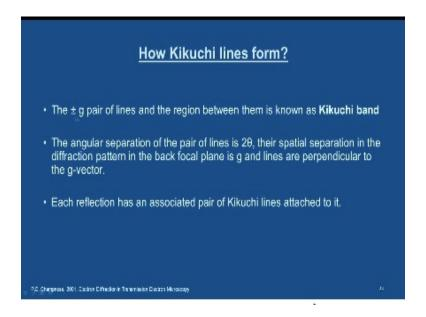
So the  $\pm g$  pair of lines and the region between them is known as Kikuchi band. The angular separation of the pair of lines is 20, their spatial separation in the diffraction pattern in the back focal plane is g and the lines are perpendicular to the g-vector. Each reflection has an associated pair of Kikuchi lines attached to it.
