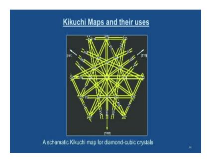
So this is the typical schematic of Kikuchi map for a diamond cubic crystal. So we will just see that some of the applications of this. You can as I mentioned that you can map the grain orientations and orientation mapping and then you can identify the faces and you can quantify all the micro structural parameters. We will just show you some glimpses of all this if not in detail.
