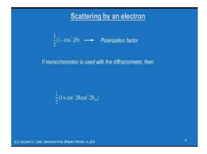
Where  $\frac{1}{2}(1+\cos^2 2\theta)$  is called a polarization factor which we will be incorporating in all the intensity equation whenever we are going to write. If monochromator is used with the diffractometer then this expression is modified into this form that is  $\frac{1}{2}(1+\cos^2 2\theta \cdot \cos^2 2\theta_M)$ .
