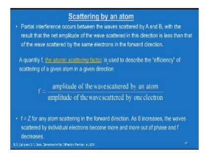
So a quantity 'f' the atomic scattering factor is used to describe the efficiency of the scattering of a given atom in a given direction, where  $\mathbf{f} = (\mathbf{amplitude} \text{ of the wave scattered by any atom})/(\mathbf{amplitude} \text{ of the wave scattered by one electron})$ . Suppose if f is equal to Z for any atom scattering in the forward direction as  $\theta$  increases the wave scattered by the individual electrons become more and more out of phase and f decreases.
