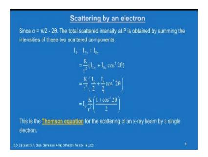
And we can look at the other expressions since  $\alpha = \pi/2 - 2\theta$  the total scattered intensity at P is obtained by summing the intensity of these two scattered components  $I_P = I_{Py} + I_{Pz}$  which we can substitute in this form  $K/r^2$  ( $I_{Oy} + I_{Oz} \cos^2 2\theta$ ) and then we can rearrange them into  $I_0(K/r^2)$  ([1+cos<sup>2</sup>2 $\theta$ ]/2). This is the Thomson equation for the scattering of an X-ray beam by a single electron.
