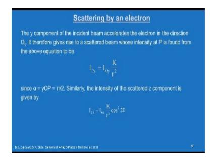
The y component of the incident beam accelerate the electron in the direction Oy. It therefore gives rise to a scattered beam whose intensity at P is found from the equation to be  $I_{Py} = I_{Oy}(K/r^2)$ . Since  $\alpha = yOP$  which is equal to  $\pi/2$ . Similarly the intensity of the scattered z component is given by  $I_{Pz} = I_{Oz}(K/r^2) \cos^2 2\theta$ .
