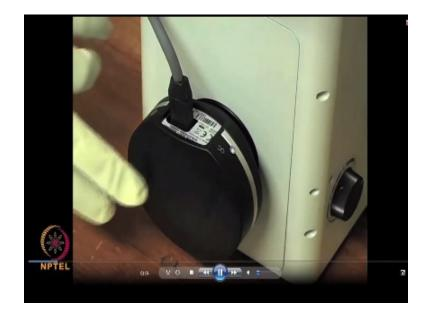
And this is a CCD camera which is being attached to this microscope and, and these are all some of the polarizing lenses.
