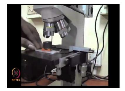
So you can see that now the specimen is being loaded in this stage specimen stage, then you choose the appropriate I mean objective lens. You can start with a lowest magnification to highest mag- you can slowly move from lowest temperature to the highest aperture. And the magnification is multiplication of these two for example you have about 5 X here and then here it is 10 so it is 50 if you choose 50 here it is 500 something like that. So here again for image grabbing,
