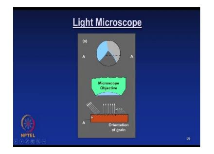
And this is just give you an introduction about this microscope you have an objective you have the specimen here; it is an is a schematic of an etched ; etched surface. And you see that light is being reflected at a different orientation because due to their different orientation of the grain. We will see actually the experiments now you can look at this references.
