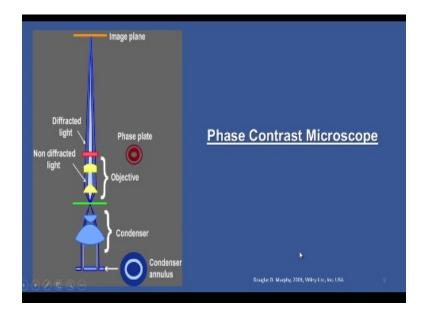
These are the similar design optical design which is shown in other reference so I will just brought it for a completion so you have the phase plate here again you have a condenser annulus here.
