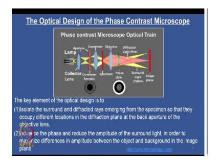
Optical design is kept In order to produce a contrast, look at this schematic you have the light source you have the aperture, lens and this is a condenser annulus like your opaque stop which I mention and then you have a condenser, specimen, objective and then a phase plate. The phase
