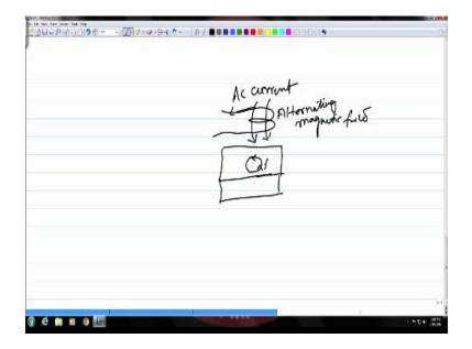
So if this carries an AC current there will be an alternating magnetic field also like this due to that alternating current which will induce this current in this conductor okay. And if there are any discontinuities around this induced current there will be change in the induced current and as a result there will be some change in this coil which needs to be detected in order to detect the defect okay.
