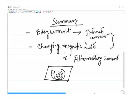
So today first we learn about the eddy current and this is nothing but the induced current on a conductive surface when you bring a current carrying conductor close to a second conductive surface okay, and the source for this eddy current as we discussed today is a changing magnetic field which comes from a changing current or an alternating current, okay.
