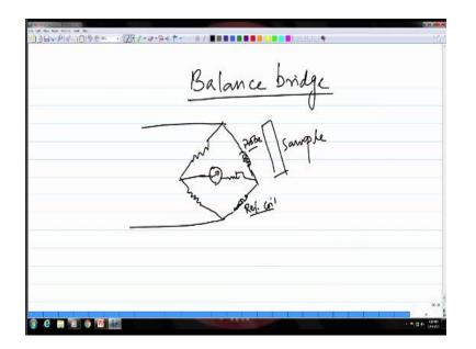
To sense the change through which you can get a signal from the defect and this balance bridge circuit or the balance bridge method is one of them through which you can sense the change the magnetic field and that is how a signal from the defect is generated and shown on the display screen of the system ok and we have also talked about the eddy current systems the different parts of it so today we will continue and see the other aspects of this particular technique.
