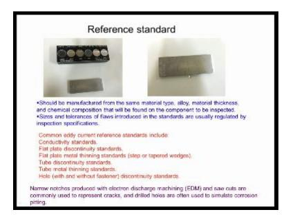
Like this so this one you have seen in the video which have this precisely cut lines which represents crack which is here also this is a conductivity reference standard because you have seen conductivity is one of the important parameters which controls the depth of penetration of the eddy currents so in certain cases you need to calibrate the instrument with regard to the conductivity as well.
