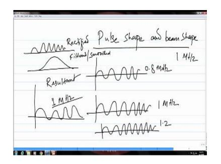
So you need an ultrasonic pulse which is generated through this transducer to send these ultrasonic waves into the sample, okay. So let us talk about that also a little bit the pulse shape and the beam the ultrasonic beam which is generated out of these pulses, so this ultrasonic waves are used in a particular frequency range as I told in the beginning and if you are selecting a particular frequency that may consist of mix of frequency which will be plus, minus to that selected frequency.
