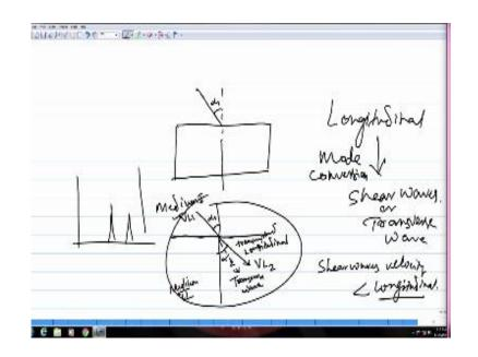
So when you send the waves are at a small incident angle so across an interface there is a possibility that if you are using longitudinal waves you there is a possibility that at the interface there will be some kind of mode conversion and a part of the longitudinal waves will be converted into a transverse wave which are also known as shear waves when the incident angle is more than zero okay.
