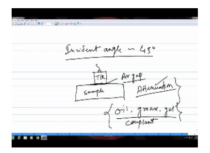
So an incident angle for this case for the steel sample which is between these two so an incident angle like 40 to 45 degree will be good in this case okay so this will ensure that shear waves are
