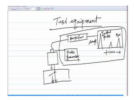
So far till last class this is what we had we first discussed about the basic principle we have learned about that and then we saw the different kinds of ultra sonic probes and then in the last class we saw this the different parts of the test equipment which is used for doing all the sonic testing okay so we will continue on this and we will see the other aspects of this particular technique.
