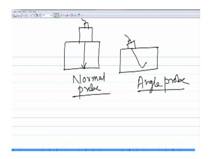
So in terms of the incident angle we saw that there are two scenarios when the incident angle is 0 then this goes vertically down like this the ultrasonic waves goes into the sample in this fashion and in some cases you need to send the waves at a particular angle like this okay because there could be cases as I would have said before also where the defects and flaws might lie at an angle or the part itself is such that you need to send the waves at some angle okay.
