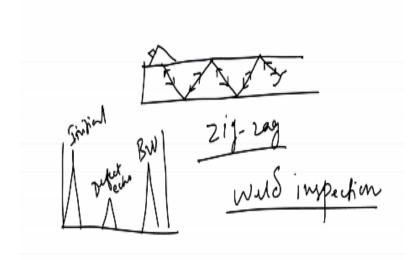
Where it is send at a particular angle what is going to happen is this is going to reflect back and forth like this, so first it will reflect from the back wall and then it is again go to the top surface and then again come back like this and so on okay so that means that back wall ECO that you see in case of a normal probe you are not going to see that in this case okay so this eco will come back only when it encounters an interface which could be a discontinuity or a defect.
