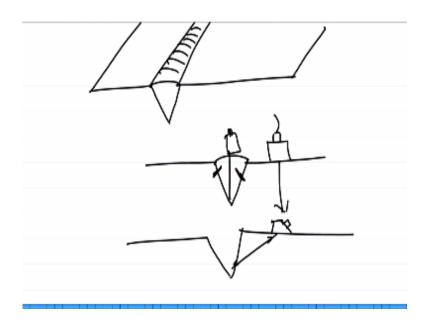
Now we are going to see a very useful application of this particular technique which is for inspecting the welds okay welding and entity they go like handing globes okay whenever you do a welding process it is followed by NDT so that you find out if the weld is sound or not if there is any welding defect or not okay and many times you would have seen a welding joint like this okay where these two plates are joint across.
