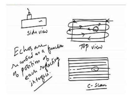
So let us say there is a defect on this sample so this is the side view of the sample and the top view is something like this, so in order to generate that plan type view of the defects you need to collect the data as I said as a function of the position of each of the reflecting interfaces and in order to do that you have to do the scan following a particular pattern like this so you have to go like this in a zigzag manner like this.
