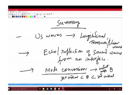
So first we learned about the basic nature of ultrasonic waves and then we saw different types of waves like longitudinal and transverse or shear then we went on to see the basic principle of this particular technique which is eco or reflection of sound waves from an interface which could be the discontinuity or the defect itself okay so then we talked about something called mode conversion when you send the waves at an incident angle a part of the longitudinal wave can convert into shared wave.
