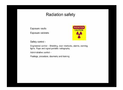
One is called the engineering safety controls and the other one is called administrative control okay. So this all is to ensure that the personal and the examiners who are working with the radiation for doing radiographic testing they are not exposed to harmful radiations okay, and at the same time people around this radiation zone are also not exposed to this radiations okay. So all these things are done in order to protect people from the harmful radiations okay.
