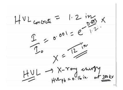
And other material which is used for shielding is concrete because you can build thick concrete walls or even the exposure chamber also in the x-ray machine can be built of concrete walls so for concrete the HVL is 1.2 inches and if you do the similar calculation like what he did just now then you will see that the thickness for which this reduces by thousand times this X will be around 12 inches okay.
