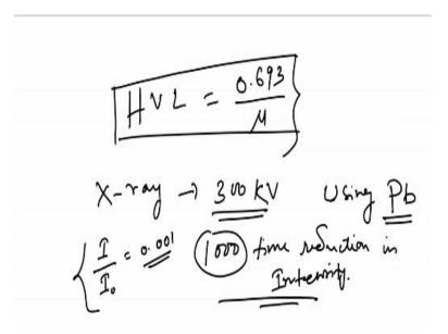
Let us take an example and then see how late or any other material can be designed to make shielding chamber based upon this half value layer for lead  $\mu$  is known and from this relationship you can find out HVL for any given material okay so let us say I have extra energy of 300 kv and I want to seal this x-ray of this kind of intensities by using lead sheets so here I need to decide what should be the thickness of lead sheet which can reduce the intensity let us say by thousand time okay.
