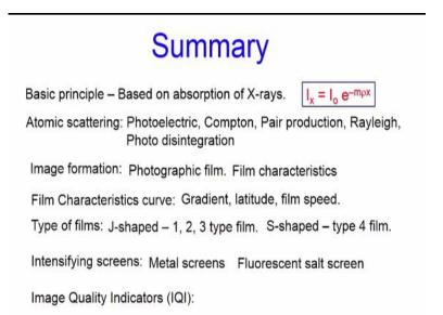
So first we saw the basic principle of this particular technique and then we learn that it is based upon absorption of x-rays which can be defined by that particular equation and then we also saw that the absorption happens due to atomic scattering events and we also learn about different types of atomic scattering like photoelectric content pair production Rayleigh scattering and photo disintegration okay.
