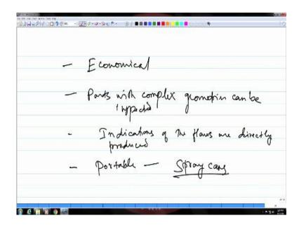
Although we have seen the dye is the main responsible factor which is going inside the flaws and things like that but even then only with the dye it is not possible to do this testing because without the developer but I will remain inside the flaws and will not come out okay.
