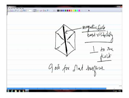
And then these slots you have so when you see the other surface the other side of this it is completely flat as I said like this. So this is what you will see on the other side of this pie gage there is no slot or anything on this surface okay. So you keep this offside down that means a slotted side will be down and then magnetize, once you magnetize and then start applying the
