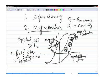
So this is what we discussed in the previous class which was about magnetizing the surface and then we saw that in terms of the magnetic field which is needed to magnetize the part you need to consider the magnetic property of the magnetic hysteresis loop of that particular material which is being tested and we saw that the applied field that should be greater than the coercivity of field HC.
