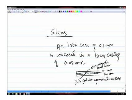
Then you have something called this is again part of the same similar kind of field indicators and these are known as shims. So it could be like a thin strip of magnetic material again which is covered by a non-magnetic material okay. For example, an iron core of 0.1mm is incased in a
