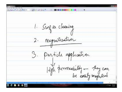
So let us see in what stage we are for this particular technique on magnetic particle testing so the first one was surface cleaning okay, then magnetizing and in this magnetization we have seen different methods and we have also learned about little bit about the theory of magnetism which is needed in this case and then you saw how a field indicator can indicate the magnitude and the direction of the field which is being applied to magnetize the part, okay.
