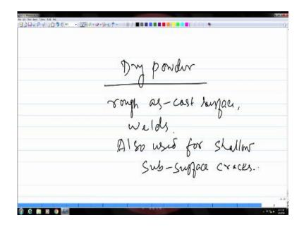
So if you talk about the dry powder it is good for rough surfaces like rough as cast surface also recommended for wells because there again you have a very rough surface as such on the weld itself if you do the inspection then the weld is very rough so there again dry particles are useful and they are also used for shallow subsurface cracks, so magnetic particle testing I should tell
