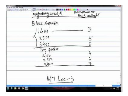
Depending on that you can say whether the magnetic current which is being applied whether that is enough or not okay. And this is how with the help of this kind of table and chart you would be able to know what should be the minimum number of particles it should be indicated for a given magnetizing current okay. And it also depends on what type of particles are used whether you are using a suspension or you are using dry powders.
