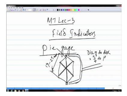
So let us continue on that so one of the field indicators we have seen but we have couple of more to talk about. The next one that we have in this is called a pie gage and this is again a small coin which is made of a highly permeable magnetic material and this coin can be divided into six or eight parts so it can be a hexagon or an octagon like this okay. So this is as big as one rupee coin made of a permeable highly permeable magnetic material okay.
