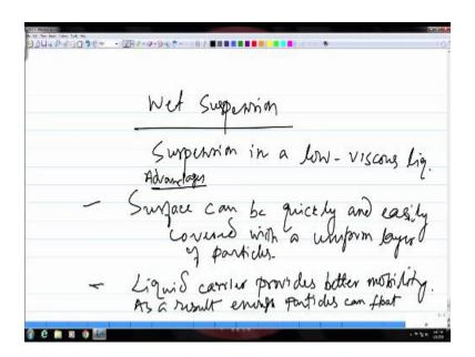
Suspension in a low viscous liquid so some petroleum liquid like for example, kerosene can be used because it satisfies the property requirements like low viscosity uniformity welding and soon, okay so that kind of petroleum liquid can be used to make the suspension and it has many advantages over dry particles as I said for example, the surface if you look at the advantages,
