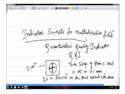
So in those cases you need the indicators which are suitable for multiple direction or multidirectional fields okay. And this kind of indicators which are used for multi directional fields are also sometimes referred as quantitative quality indicators or QQI in short okay. So that means in this case you need some feature on the indicator which can indicate the direction of the field in different directions okay.
