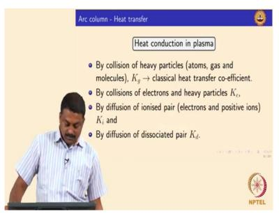
Can happen by four ways again the first one is classical way by collision of heavy particles by collision of atoms gas molecules okay that means that if a one particle which is hard is collided with the other one obviously heat is transferred from one place to another. So that is the classical heat transfer coefficient case it happens in conductors for example in copper rod, okay.
