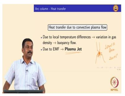
So then heat the third heat transfer mechanism is convective flow. And this is also significant how the heat is transferred from one place to other place in arc okay there are two ways the heat is transferred becomes convective heat transfer. So one is very simple buoyancy law what is buoyancy flow again? Because of because of density difference gas is at high temperature will be less tense than the gases at low temperature and that will lead to a buoyancy flow isn't it?
