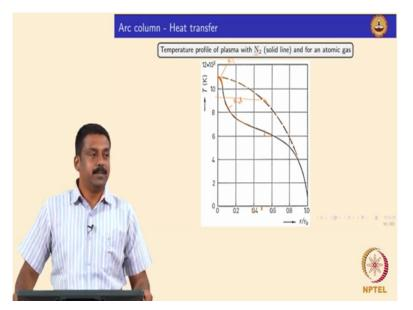
For example this is a temperature profile of an arc neglecting radiating radiation convective heat transfer so we have calculated temperature profile of a plasma with diatomic nitrogen and a mono atomic nitrogen gas. And what we see over here it is RBR zero R zero is the radius of an arc at any given location if it is centre that means it will become zero right or becomes U.
