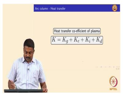
Okay so the total K of an arc is nothing but KG but it is a classical heat transfer coefficient by the collision of heavy particles atoms and molecules and then the collision of electrons and (())(8:19) heavy particles the electrons carry huge amount of heat they also have a much higher drift velocity and they determine the electric current in an arc we just saw. Isn't it?
