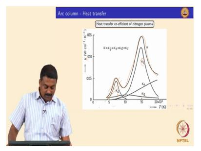
How? Like this so this is the total a coefficient heat transfer coefficient by conduction so KD what is the term dissociation de dissociation that can be significant lower temperatures okay and high temperature yeah deionization okay KE is collision of electron with heavy particles and then KG is the classical heat transfer okay by the collision of atoms and molecules if we sum it up this how the distribution looks like.
