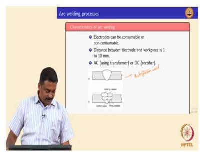
In a typical characteristics welding you can either make the electrode consumable or non consumable okay so generally the distance between the tip of the electrode to work piece not more than 10 mm otherwise your arc stability decreases significantly because then the conduction, convection, radiation it becomes extremely unpredictable okay because the current density is distributed much over distances okay.
