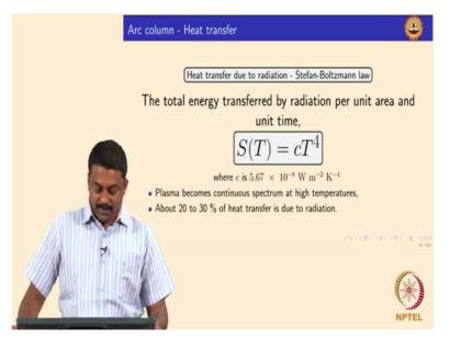
So here so if you assume the arc is a continuous spectrum there is a black body so once you assume that obviously at high temperature DD is a continuous spectrum if temperature is low then only you get line spectrum then this equation is not valid okay so plasma becomes continuous spectrum at high temperatures.
