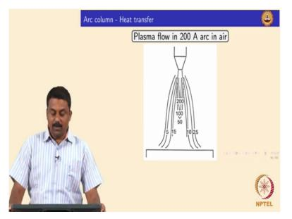
Plasma flow it is just a simple toned amperes arc in an arc. So the centre so this is your electrode the flow close to the electrode can go as high as 200 meter per second. And if you go far away in the arc envelope the envelope side you don't have the accumulation isn't it? Of the charges, charge recommendation always happens either at cathode or anode.
