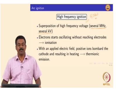
So the third method which is very popular which commonly used for arc ignition is by highfrequency ignition, so what we do is in this case we just apply the high-frequency electric field okay several megahertz and sometimes we also use it but most commonly used is use high frequency current and when you apply high-frequency current the electron would not reach the end would because your loss would be changing the polarity in most of the cases okay.
