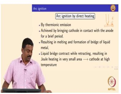
We ignite the arc by direct heating, so just strike an arc by touching cathode anode which is not that straightforward okay, so if you keep on touching it you will not strike an arc okay, so you need to retract the electrode slowly, so then you can strike an arc okay, so it is done by thermionic emission because the moment you have an arc circulating, so then you will have actually heating, triggering the heating of the system okay.
