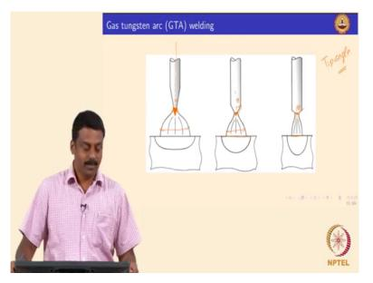
The other important characteristic of electrode is electrode tipangle, it is very very important okay, in most of the industrial production conditions and this is very significant because you may start with emissioning the electrode in the morning they were stiffed rods, so when you keep mould welding it without change emissioning the tip again, you would significantly the bid geometry okay.
