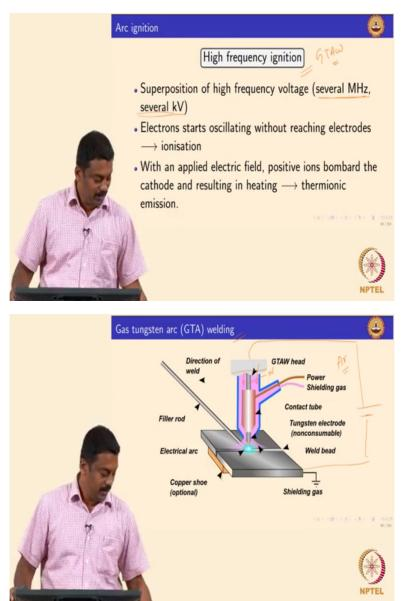
Okay, now will move on to the main process, the gas tungsten arc welding so we look that the physics of arc and we ignited the arc, now we can weld right, so if you look at the gas tungsten arc welding, it is one of the simplest processes, so all we are to do is we need to ignite the arc and then we can weld, so will have in the setups, so this is the base material okay, so sometimes we also use an copper backing plate, backing plate to conduct the heat
