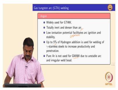
So will look at the one by one all the characteristics of the gases than we will stop okay, the first argon, so argon is widely used for GTAW, it is totally inert and denser than air, it is very important, so when you use argon shielding gas it displays the air okay, so the air is displaced effectively well-organised perched because it is denser than air, so it has very low ionisation compared to helium okay.
