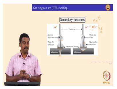
So these what happens when you have an argon Ar CO2, so the arc core is very narrow in argon case because the heat is not transferred, so there is no conductive heat transfer, there is no de-dissociation, other the conductive heat transfer by de-dissociation, so you will concentrate heat at the core the maximum when you use a pure argon right, so you will have very narrow core and leading to the deeper penetration in argon.
