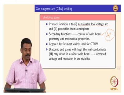
So now will move on to the shielding gases shall we right, so we looked at the heat transfer characteristics right, the conduction conversion radiation, so it is recover all the time, so the moment when you see the selection of gases whatever we learned in the heat transferred is extremely important to relate that over the correspond shielding gas okay, so the function of gas in the welding process primary function is to strike an arc is not it.
