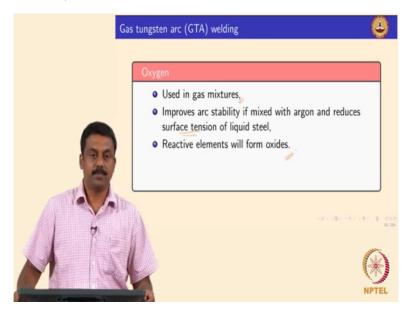
Look at two more gases and then we stop oxygen, so oxygen is always used in mixture you cannot do and welding with pure oxygen for obvious reasons, so you will have explosion right, so it is use widely to mix pure argon, mostly argon okay, so it is known to improve the arc stability right but again you have diatomic oxygen O2 would lead to de-dissociation and the spreading and it will also influence the surface tension okay.
