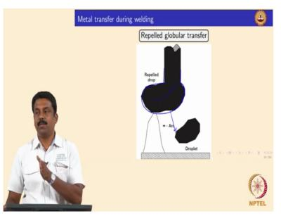
And if increase the current slightly further it becomes repelled, okay so repelled acts on the globular shape changes to repelled globular because of the increasing current so there will be
