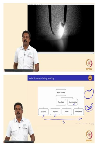
So based on the force balance you may have the droplet transferred in various modes. In most of the cases the diameter of the droplet and the frequency of droplet transfer will determined by which force is rate controlling? If gravity is rate controlling, droplet will be transferred with high mass like a globes the volume will be higher, if Lorentz force is rate controlling it can transfer very small diameter (())(0:47) droplet at much higher frequencies, why? Because melting rates, okay.
