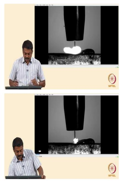
I will show you video, it will be very clear. So this is transfer, so what is happening here? So you have an arc so transfer happens by short circuiting and during the short circuiting event there is no arc, do you see that so you establish a arc with the arc length and then you switch OFF the arc the moment the short circuiting happens and then you transfer the droplet by the surface tension of the liquid pool, is it clear?
