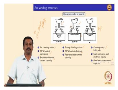
And before that I have already explain this, the polarity. The effect of polarity, you can either make your (consu) electrode positive or negative, so in first case we have electrode is negative, if electrode is negative what will happen? The ions would go and accumulate, ok. So if this is negative electrode negative, so the ions would travels towards electrodes and then electrons will travel towards.
