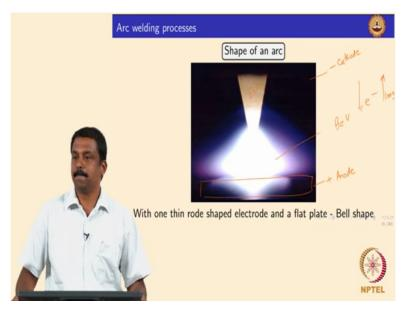
So whatever I have explain this discharge it is sustained inside the these guy the white bright regions, so the continuous discharge leading to collision of the energy carriers. What are the energy carriers in this case?
