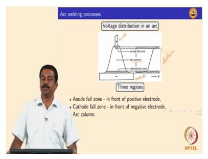
So what is important here if you want to understand how the heat is generated? We need to look at what are the component inside the arc, say I already explain you can make either the electrode positive or negative, ok does not matter whether you want to melt the electrode or you want to keep the electrode say for long time. Suppose assuming if we make the electrode positive and the work piece negative, so which is cathode here?
