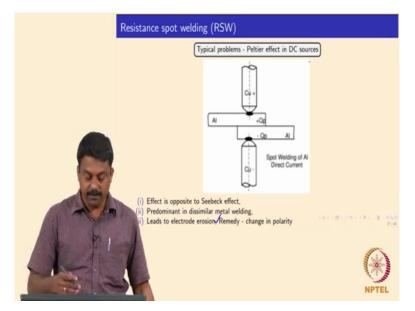
And then the Peltier effect, right? So you will expect an electrode erosion very severe electrode erosion and because of the dissimilar heating.
