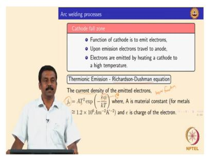
So the main function of cathode is to emit electrons, ok it is very important. So the function of cathode is extremely important because that is where you emit electrons, so once you emit obviously it will travel to the electron will travel to the anode but during this process it will also interact with the medium gas causing some more emissions, the avalanche, the discharge, ok.
