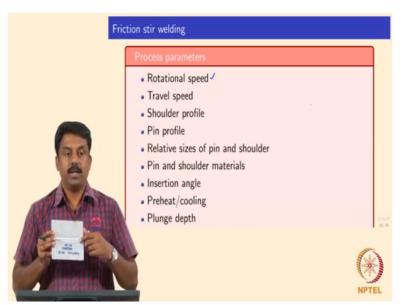
the speed of rotation, travel speed, the shoulder profile and the ratio the size between the pin and shoulder.
