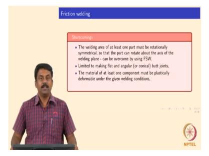
The other major advantage is low labour cost, good so we will move on, so what are the disadvantages? See there must be some symmetry, isn't it? In frictional stir welding so if this rod, if this rod is slightly larger than the other rod, diameter is larger, and it is very difficult to weld, isn't it? So, you will not achieve, it's very difficult unless you do an angular weld or orbital weld, so you need some symmetry at the interface.
