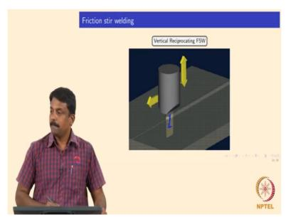
So, the other variants, instead of a linear reciprocating motion you also have a vertical reciprocating motion, okay, you still have the blade instead of going linear way, so you also have vertical, going up and down, isn't it? And this can also cause heating at the interface, so the clamping of the plates enables mechanical deformation across the interface and you end up making a joint. Yes, it's clear? So ultimately all the process parameters are important what I talked about, okay.
