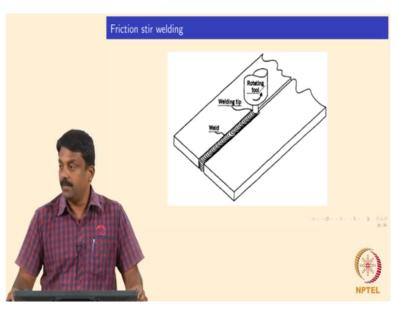
So, we also brought some sample, we look at it after looking at the slides, so this is clear, right? A rotating tool is actually plunged onto the sample and then that material is deformed at the interface during this process, so its high temperature enables easy flow of material, mechanical behaviour of material, okay because material softens at high temperature.
