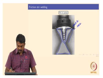
Okay, so we will move onto next so this is the pin in action so one of the pins what you see over here so pin profile and you have a shoulder here, okay, and then this is the pin and this rotating along clockwise so if it is clockwise you have advancing side and retreating side and you see the depth is not controlled so in this case we are doing it in both sides so this is the bottom side and this is top side, right?
