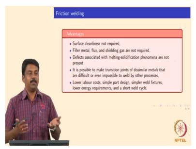
So, in Frictional welding in general what are the advantages compared to the arch welding, it's not only friction, Frictional stir so the biggest benefit of friction is surface cleanness
