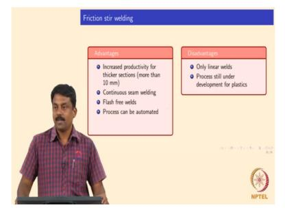
Okay, we will move on to the some of the theories and then we will move to the next welding process, right? So frictional stir welding, what are the advantages? So main advantage of friction stir welding is in my opinion, so you can weld softer material I mean material which can flow easily, right, material which softens easily with the temperature, okay so Aluminium alloy, it softens significantly when the temperature is increased. So, right?
