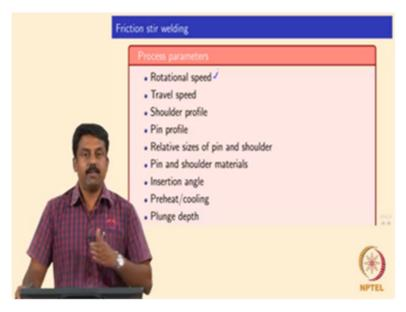
And then the process parameters we looked at last class is rotational speed that's RPM of the tool itself, the welding speed or the travel speed and the shoulder profile, pin profile, okay and the relative size of the pin to the shoulder, that will all influence the flow of material as well as the frictional heat generation.
