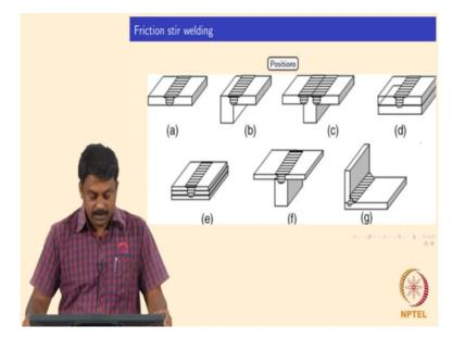
So, what are the positions that can be welded using frictional stir so one of the major disadvantage of frictional stir welding so the accessibility, okay, so you cannot same as resistance pot welding, you cannot weld it when you can't access the joint with a pin and shoulder, isn't it? So, you need a reasonable accessing otherwise how are you going to insert a shoulder and a pin and then make linear weld?
