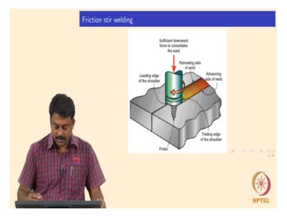
So now so there are some distinctive regions along this weld interface and we looked at this slide in in last class. So, when a tool is rotating along this direction, so we have an advancing side and retreating side, okay, so if it is rotating like this so you have advancing side and retreating side, isn't it?
