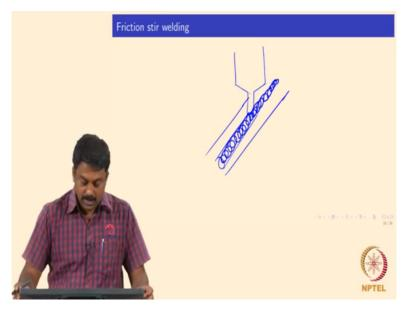
Okay so in Frictional stir welding, if you look at so the important process parameters say we looked at the shoulder itself and the pin so I am just drawing a very simple sketch of frictional stir pin and the interface to be welded so it is actually somewhere over there so pin is actually inserted onto the interface and then you make a mechanical deformation, isn't it? So, this mechanical deformation happens from one interface to other interface creating a joint at the interface.
