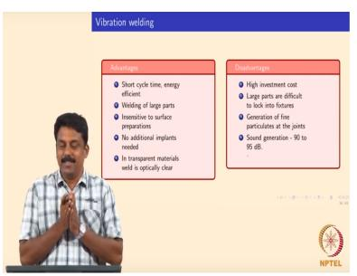
Again advantages again, so this are very important to select a welding process, so what are the advantages vibration welding it is short welding time and then the efficient make a huge a larger
