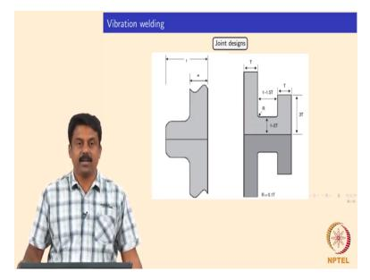
So joint design so the symmetry should be maintained so to otherwise you dissipation can be very tricky in vibrational welding.
