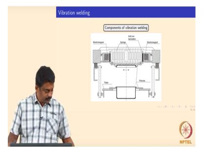
So this is a sematic so this is a container to be welder so another dimension object, so the bottom what is fixed within vicious the top is mounted with electromagnetic vibrations in it this been attached and this part goes in there and this vibrates in this case linearly a top and then subsequent I mean after appoint heating the interface then you also applied downward force and then the two parts can be joint is it clear good.
