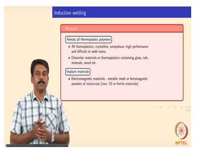
So material so almost all thermoplastic material crystalline, amorphous on high performance difficult to joint and the all can be weld resins in induction welding, so dissimilar materials or thermoplastic containing glass talc minerals wood they all can be weld in the implant material generally it is electromagnetic material generally we use as an metallic mesh ferromagnetic micro mesh is resent in to the inside the implant alright it is clear.
