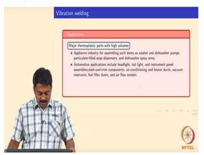
So what are the applications of these, so the high volumes so mainly appliance industry like for example for water bottles washer and dishwasher pumps soap dispensers dishwasher spray arms for example, so (())(19:09) is not very rarely used yeah either vibrations welding or ultrasonic
