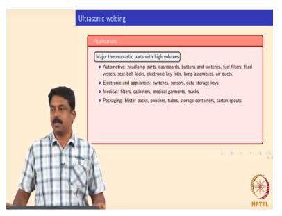
So we will move on to the application and then we will look at that as a bounding, so ultrasonic welding so what are the application automotive applications the majority of parts plastic parts
