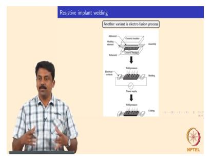
So instead of using induction we can also resist this current the same principle you are saying resistive implant welding you are heating up the implant the resistance heating so in the advantage of these process is in the implant may not be dope with material, so what we need we use an induction coil replace the implant on top of coil melt the implant and subsequently you can take the induction where out.
