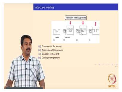
So this is an induction welding process the first to place in implant and you have work while and this two surfaces to be joint, so this is top and this is bottom implant is place and the induction coil send the electromagnetic ways and during this process we implant heats up and then you apply a down work force and then implant melts and joints center-face subsequently the implant can be solidified it is clear induction welding process.
